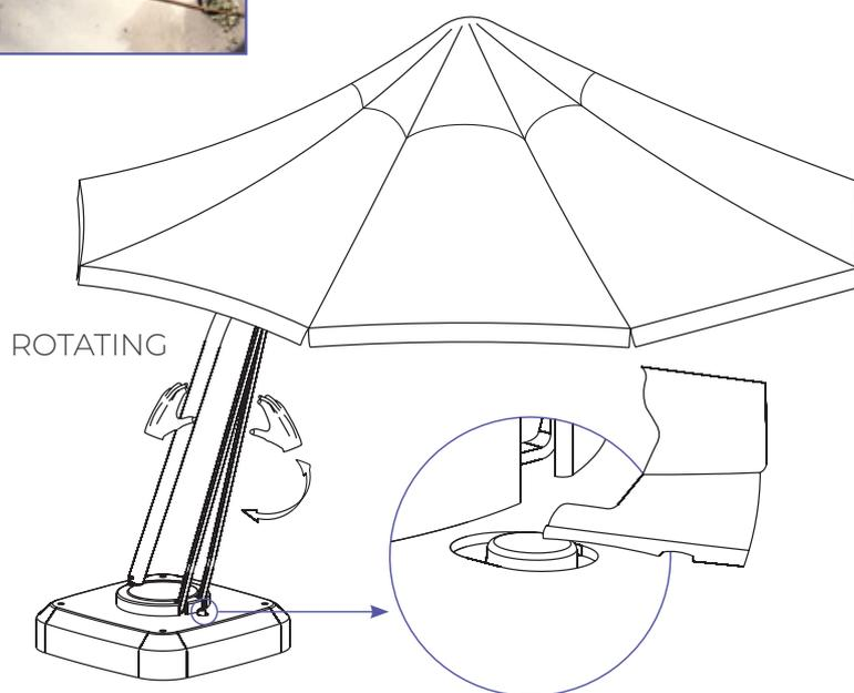
2. **Screw wells with wheels** – The screw wells come with round plastic caps which prevent water from entering them. If these caps are not kept on top of the wells, water and moisture collects inside the wells, causing them to rust. Do ensure the plastic caps are always in place to prevent this.
